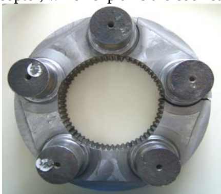
Fig. 3. Carrier Plate with five cracked posts.
