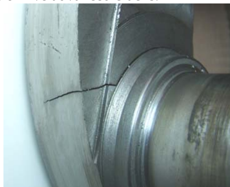
Fig. 4. Carrier plate #1 post crack
