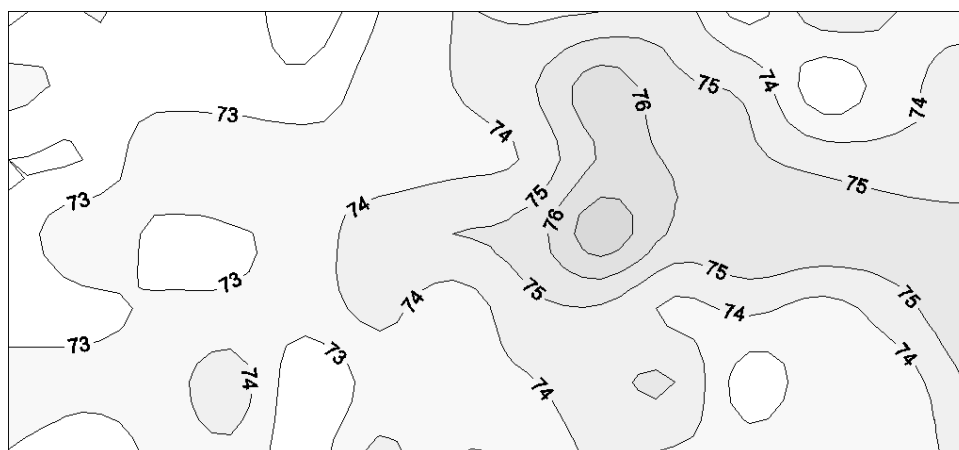
Figure 1 – Sound level distribution in the compressor room –Variant I
