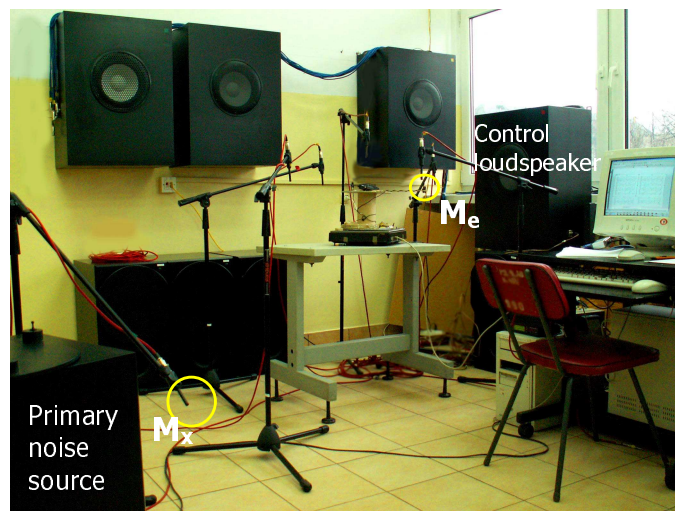
Figure 1 – ANC system for creation of 3D zones of quiet in enclosure.
