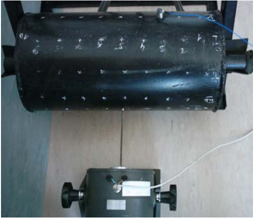
Figure3 – The cylinder mechanically excited by a shaker.
