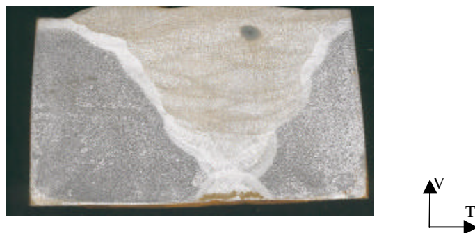
Figure 3 –macrograph of the automatic welding in the plan (TV).
