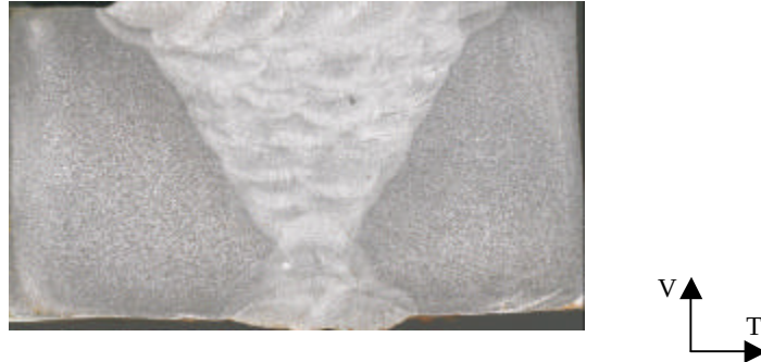
Figure 2 –macrograph of the manual welding in the plan (TV).
