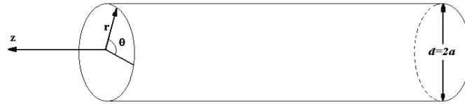
Figure 1 - The coordinate system used in the derivation of equations.
