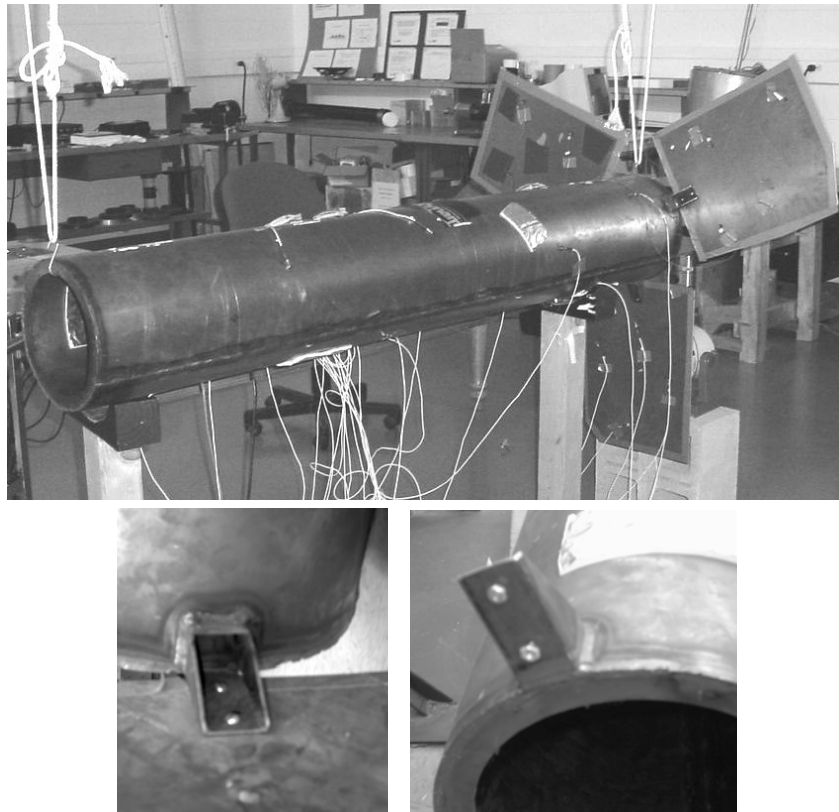
Figure 1 – Cylinder-plate structure: the top picture shows the experimental setup with the lower plate driven by a shaker (point force); the bottom pictures show details of the bracket junction and cylinder end.
