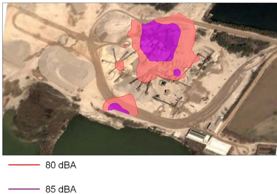
Figure 3. Noise contour map (80 and 85 dBA) in gravel pit II.
