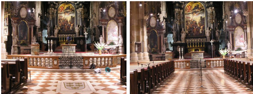
Figure 3 - Measurements at the cathedral: the source was located at the Volksaltar and the microphones are in the Hauptschiff
