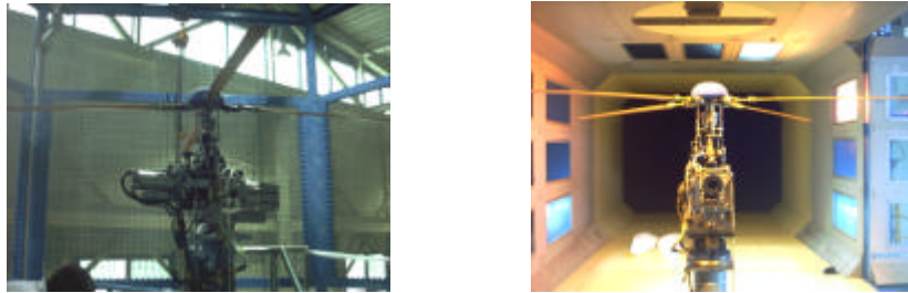
Figure 6 – Test Rotor Model installed in KARI GSRTS (left) and in KARI LSWT (right)
