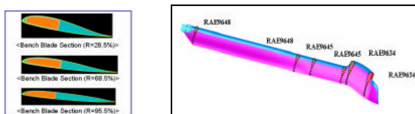
Figure 4 – Blade sectional construction of advanced tapered blade
