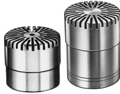
Fig. 5 The frequency response of the half-inch Reference Microphone (right) is essentially flat due to its highly tensioned diaphragm and its large internal cavity
