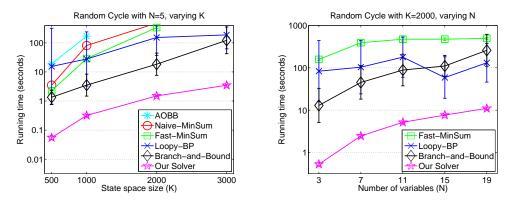
Figure 2. Comparing Cycle Solvers. Note that time axis is in log scale. AOBB is AND/OR graph branch-andbound (Marinescu & Dechter, 2006). Naive-MinSum is the naive way of passing clique tree messages. Fast-MinSum is algorithm 2 in (Felzenszwalb & McAuley, 2011). Loopy-BP is loopy min-sum message passing. Sometimes it takes extremely long to converge, especially for short cycles. We always cut it off at 500 seconds. Branch-and-Bound is the method of (Sun et al., 2012).
