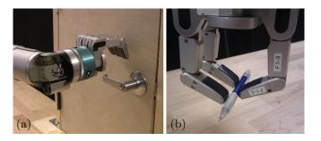
Figure 1. Force control policies for two different manipulation tasks were learnt using our method: (a) opening a door, and (b) picking up a pen from the table.
