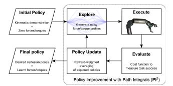
Figure 2. A high-level overview of our approach to learning force control policies for robotic manipulation.
