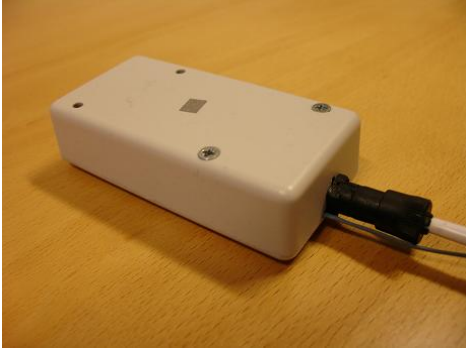
Figure 1. Sensor-actuator device consisting of motion sensor hardware and a vibrotactile actuator C2.
