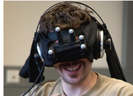
Figure 1: Equipment of one subject. The subjects wear AR goggles, headphones and cloth to ensure that they do not bypass the goggles.
