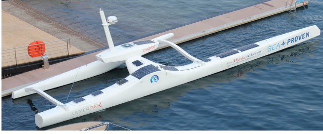
Fig. 1. The ASV Sphyrna, 17m long, Polynesian design.
