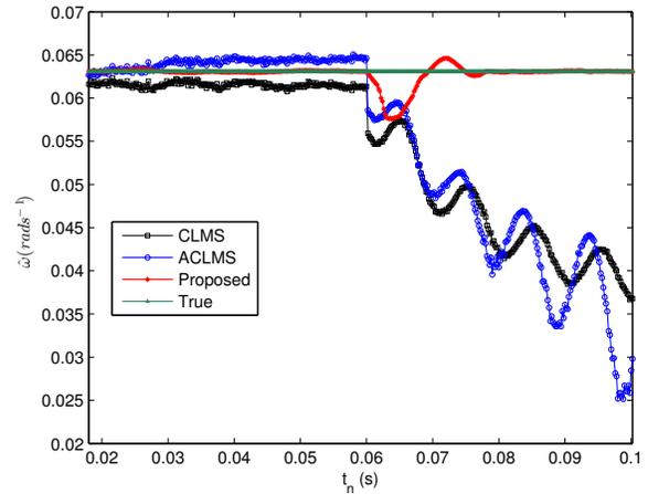
Figure 4. Frequency estimates in unbalanced system
