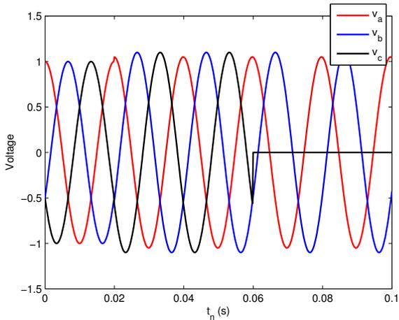
Figure 3. Three channel signals in unbalanced system
