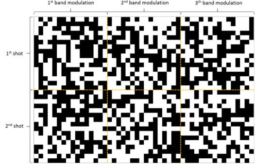
**Fig. 3.** Proposed  $\mathbf{X}$  matrix arrangement of a colored coded aperture in binary representation to modulate a spatio-spectral data cube of dimensions  $16 \times 16 \times 3$ , and for 2 snapshots.
