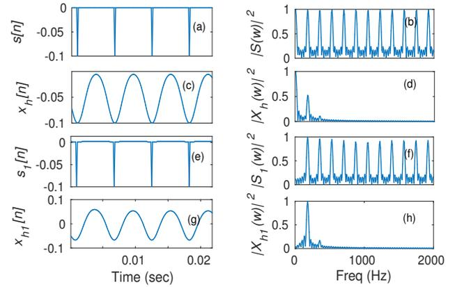
**Fig. 2.** (a) Synthetic impulse sequence ( $s[n]$ ). (c) Filtered signal  $x_h[n]$  ( $x_h[n] = s[n] * h[n]$ ). (e) Local mean subtracted signal ( $s_1[n]$ ) of the impulse sequence  $s[n]$ . (g) Filtered signal  $x_{h1}[n]$  by ( $x_{h1}[n] = s_1[n] * h[n]$ ). (b), (d), (f), and (h) show the magnitude spectra of (a), (c), (e), and (g), respectively.
