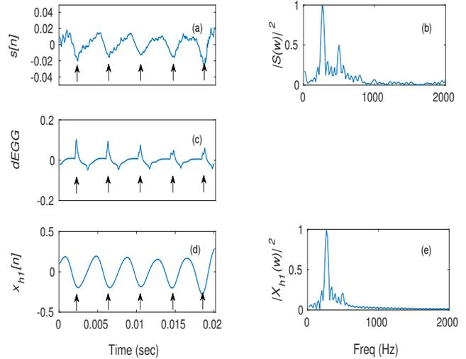
**Fig. 5.** (a) Speech signal segment  $s[n]$  of a female speaker's neutral speech (voice bar /b/). (c) dEGG segment corresponding to  $s[n]$ . (d) Filtered segment  $x_{h1}[n]$  using the two filter operations. (b) and (e) Show the magnitude spectra of (a) and (d), respectively.
