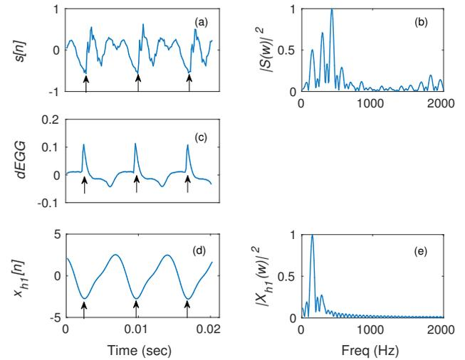
**Fig. 3.** (a) Speech signal segment  $s[n]$  of a male speaker's neutral speech. (c) dEGG segment corresponding to  $s[n]$ . (d) Filtered segment  $x_{h1}[n]$  using the two filter operations. (b) and (e) Show the magnitude spectra of (a) and (d), respectively.
