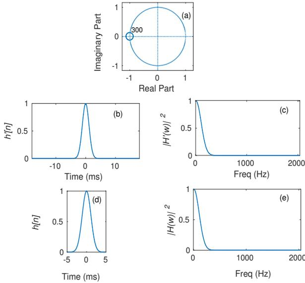
**Fig. 1.** (a) Pole-zero plot of the proposed filter. (b) Impulse response ( $h'[n]$ ). (c) Magnitude spectrum ( $|H'(\omega)|^2$ ) of the filter. (d) Truncated impulse response ( $h[n]$ ). (e) Magnitude spectrum ( $|H(\omega)|^2$ ) of the truncated impulse response. Note: The magnitude spectra are amplitude normalized by dividing with respective to the maximum values.
