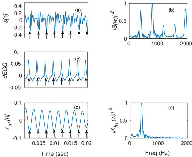
**Fig. 4.** (a) Speech signal segment  $s[n]$  of a female speaker's angry speech. (c) dEGG segment corresponding to  $s[n]$ . (d) Filtered segment  $x_{h1}[n]$  using the two filter operations. (b) and (e) Show the magnitude spectra of (a) and (d), respectively.
