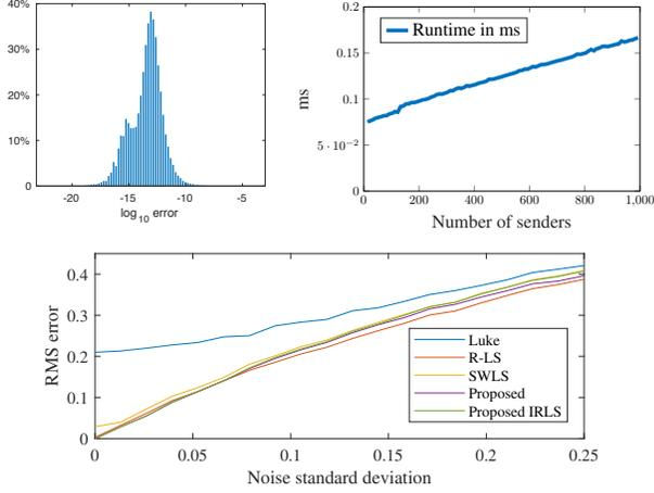
**Fig. 2.** *Top left:* Distribution of errors for synthetic noise-less instances. *Top right:* Runtime (in ms) for different number of senders. *Bottom:* RMS error in receiver position for various amounts of noise.
