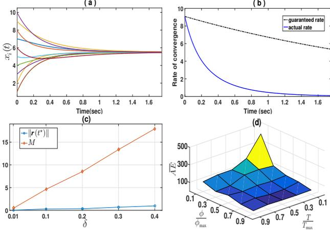
**Fig. 3:** (a): Average consensus for  $x_i(t)$ , (b): Convergence rate, (c): Actual ( $\|\mathbf{r}(t^*)\|$ ) and max. quantization error ( $M$ ), (d): Average no. of events  $\overline{\text{AE}}$  versus  $\{T/T_{\max}, \phi/\phi_{\max}\}$ .
