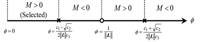
**Fig. 2:** Operational range for  $\phi$  for guaranteed convergence. ‘x’ and ‘o’, respectively, denote the poles and zeros of  $M$ .
