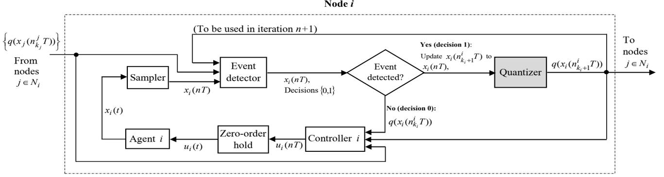
**Fig. 1:** Proposed Q-CEASE for node  $i$ , iteration  $n$ , and the previously quantized event  $q(x_i(n_{k_i}^i T))$ . Compared to implementation [15], the shaded quantization block adds an additional level of complexity.
