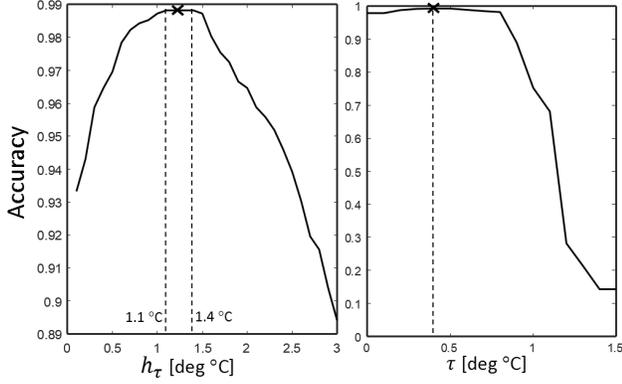
**Fig. 3.** Optimized threshold  $\tau$  and body induced thermal signature  $h_\tau$  for typical 3 m ceiling mounted sensors.
