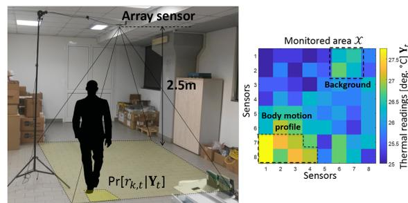
Fig. 1. Layout example and noisy temperature readings.
