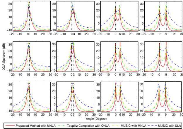
**Fig. 2.** Angle resolution comparison for different SNRs and different angle separations between sources  $\Delta\theta$ . SNR is set as  $-5$  dB,  $0$  dB, and  $5$  dB (from row 1 to row 3), and the angle separation  $\Delta\theta$  between two sources is set as  $2^\circ$ ,  $3^\circ$ ,  $6^\circ$ , and  $9^\circ$  (from column 1 to column 4).
