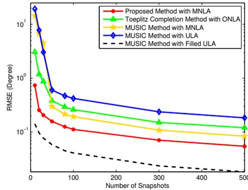
**Fig. 4.** RMSE versus snapshot number with  $\text{SNR} = 10$  dB.
