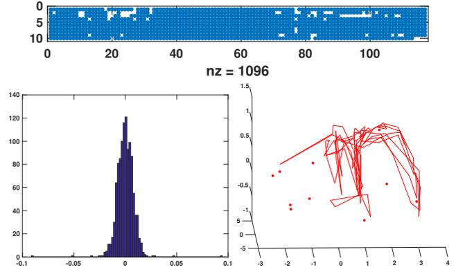
**Fig. 3.** For the cave experiment the figure shows detected inliers  $W_{in}$  (top), inlier residual histogram (bottom left) and estimated microphone and sound source positions, red dots and line respectively (bottom right).
