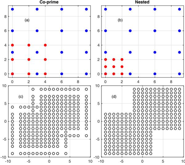
**Fig. 1.** 2D Sparse arrays: Examples of (a) Co-prime and (b) Nested arrays along with their difference coarrays in (c) and (d) respectively. For the physical arrays in (a) and (b) the two colors correspond to the two subarrays which make up the sparse array.
