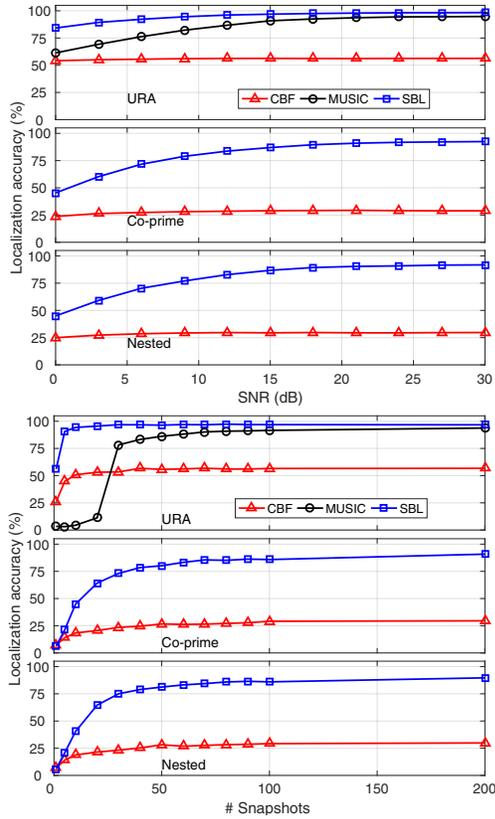
**Fig. 3.** 2D Beamforming: Percentage of sources localized over 100 Monte Carlo simulations for changing SNR (top) and changing snapshot number (bottom). All the arrays have same aperture, number of sources is  $K = 25$ .
