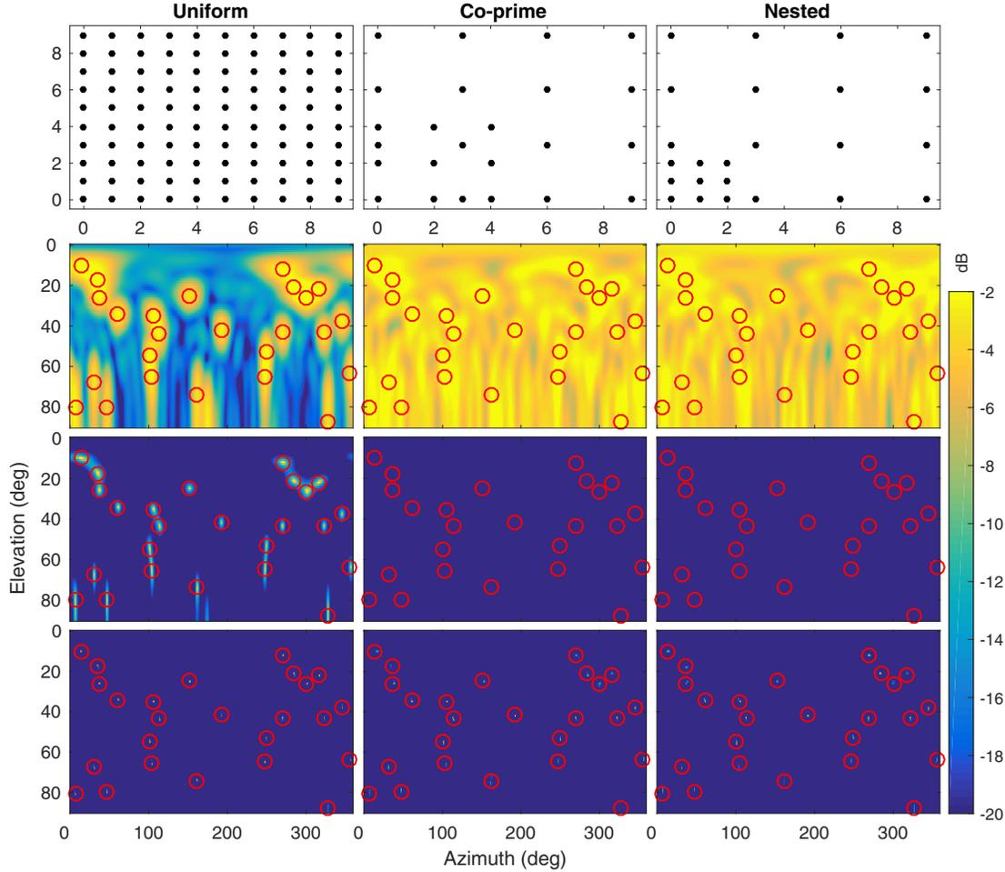
**Fig. 2.** Sensor positions for various 2D planar arrays (top row). Estimated 2D spectrum when  $K = 25$  sources are present using CBF (second row), MUSIC (third row), and SBL (last row). Circle ‘o’ indicates true source positions.
