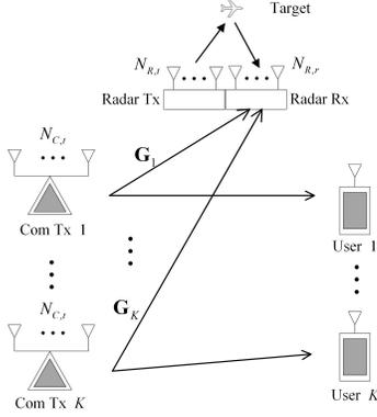
**Fig. 1.** Diagram of joint radar-communication co-existence system.
