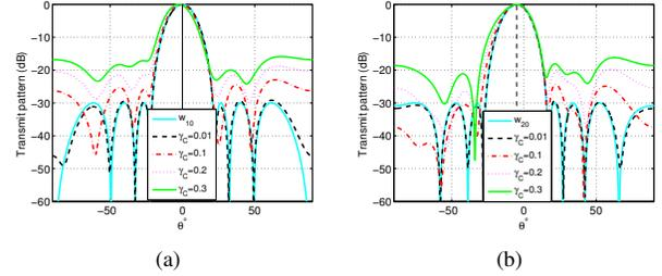
Fig. 4. The transmit beampattern behaviors for communications with  $\gamma_R = 0.3$ . (a)  $\mathbf{w}_1$ , (b)  $\mathbf{w}_2$ .
