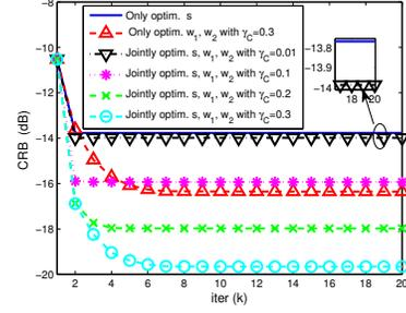
Fig. 2. The values of objective function versus the iteration number with  $\gamma_R = 0.3$ .
