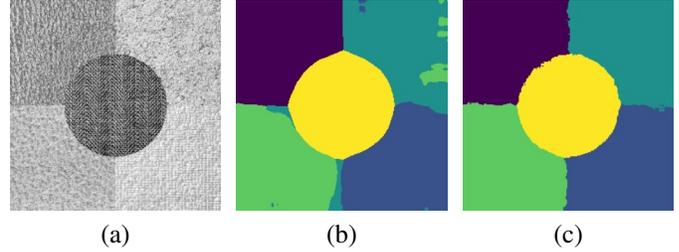
**Fig. 1.** Segmentation results step by step. (a) A texture mosaic with 5 different components from Brodatz texture dataset. (b) Raw segmentation results with proposed PRP features. (c) Final segmentation mask after post-processing.
