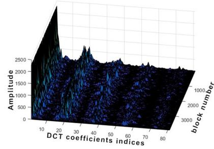
Fig. 4: Cluster structured sparsity of the DCT coefficients of natural images.
