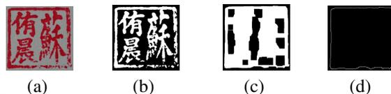
**Fig. 2:** The contours detected on the imprints. (a) The seal imprint image with the name “蘇侑晨” captured using a camera. (b) The binarization result of (a). (c) The image after the process of morphological operations. (d) The contour identified from (c).
