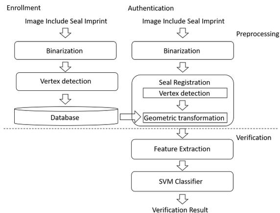
**Fig. 1:** Process flow for the proposed system
