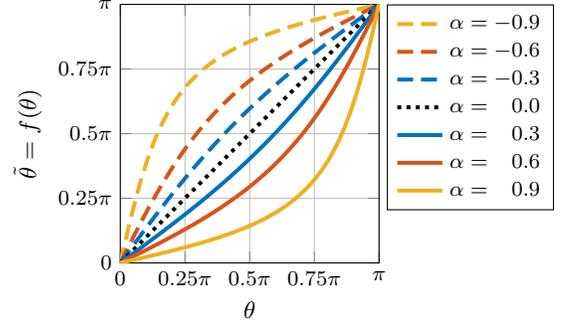
**Fig. 1:** Exemplary space warping function from Eq. (14) with variants of the warping factor  $\alpha$ .
