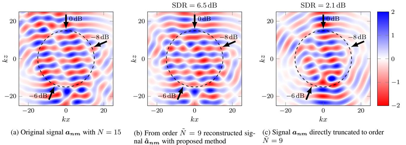
**Fig. 2:**  $xz$ -planes of sound field snapshots corresponding to different HOA signals. All HOA signals represent three plane waves impinging from the indicated directions with amplitudes as labeled.
