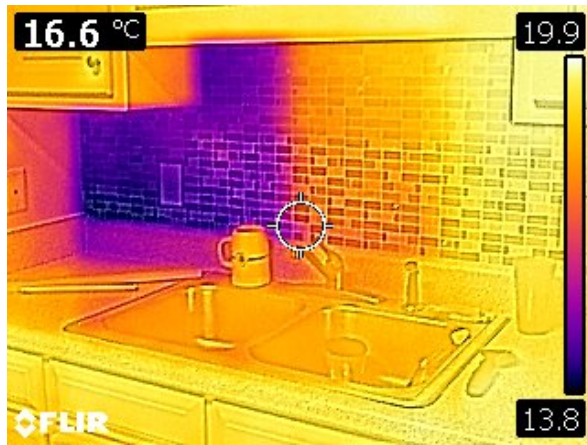
Fig. 2: An example IR image, with MSX image fusion. The image shows a kitchen backsplash on a wall with a poorly insulated fire-place behind it. The dark area in the upper left of the image indicates a colder region, due to insufficient or missing insulation.
