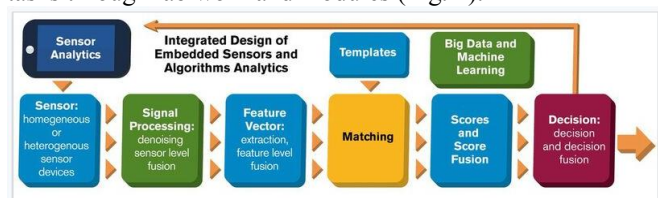
Fig. 1 Integrated sensor device design and algorithm development. Algorithms include denoising, feature extraction, machine learning and fusion.
