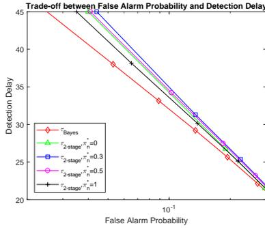
**Fig. 1.** Comparison of trade-off performance for the optimal stopping time  $\tau_{\text{Bayes}}$  and naive stopping time  $\tau_{2\text{-stage}}$  with different nuisance change threshold  $\pi_n^*$ .
