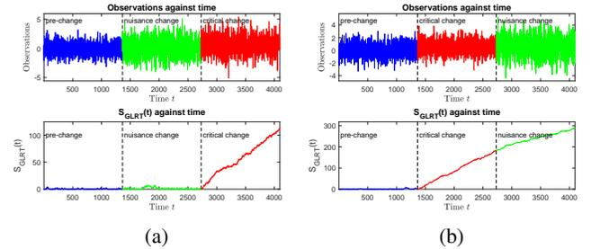
**Fig. 3.** Examples of  $S_{\text{GLRT}}(t)$  values with different choices of  $\nu_c, \nu_n$ . (a)  $\nu_c = 2730, \nu_n = 1365$  (b)  $\nu_c = 1365, \nu_n = 2730$ .
