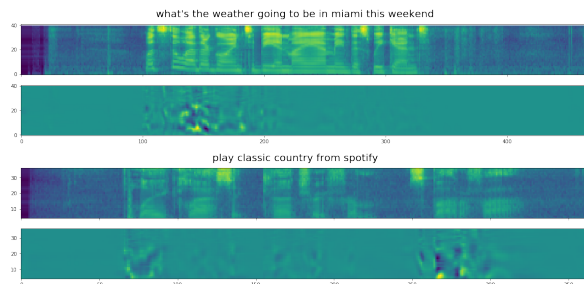
Fig. 5: Filter-bank features and corresponding saliency maps for our speech-to-domain model. It can be seen that the model responds to “what’s the weather” part and “play” or “spotify” from the second example. Top image is “weather” domain, bottom image is “music” domain.
