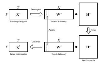
Fig. 1. Basic approach of NMF-based voice conversion
