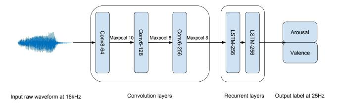
**Fig. 1**. The proposed convolutional recurrent neural network for speech emotion recognition. A CNN is used to extract features from the raw signal before feeding them to a 2-layer LSTM network for the final prediction.
