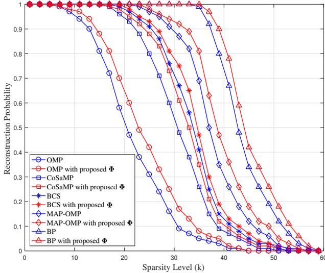
**Fig. 2:** Reconstruction probability versus sparsity level for a randomly generated binary signal (Bernoulli process) with noise-free measurements using the parameter set  $\{n = 120, m = 250, L = 12, \ell_{inc} = 2\}$ .
