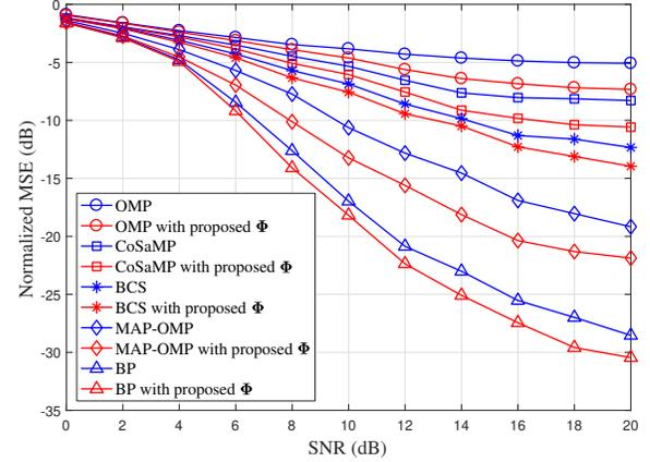
**Fig. 3:** Normalized MSE versus SNR (dB) for the randomly generated Gaussian signal using the parameter set  $\{n = 120, m = 250, k = 30, L = 12, \ell_{inc} = 2\}$ .
