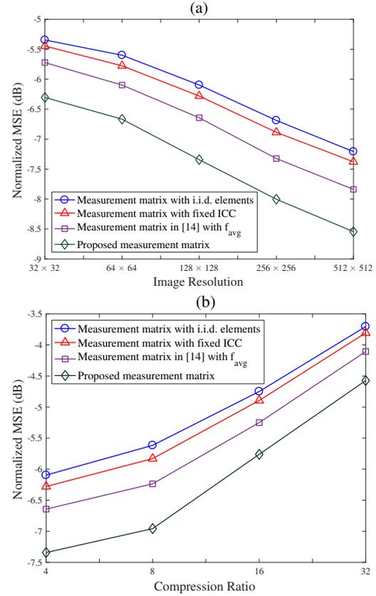
**Fig. 4:** (a): Normalized MSE versus image resolution for a compression ratio of 4, (b): Normalized MSE versus compression ratio for images of resolution  $128 \times 128$ .
