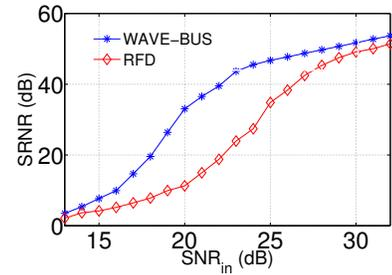
**Fig. 5.** SRNR for WAVE-BUS and RFD methods versus  $\text{SNR}_{\text{in}}$ .
