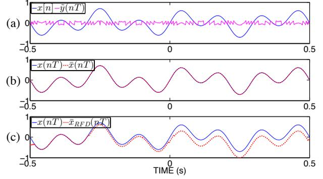
**Fig. 4.** Unlimited sampling in the presence of noise ( $\text{SNR}_{\text{in}} = 20$  dB and  $\lambda = 0.05$ ): (a) The signal  $x(nT)$  and its noisy modulo samples  $\tilde{y}(nT)$ . Reconstructions using (b) WAVE-BUS and (c) RFD methods with reconstruction errors at  $-80$  dB and  $-7$  dB, respectively.
