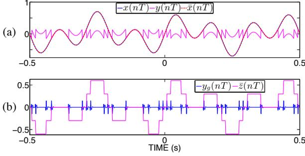
**Fig. 3.** WAVE-BUS with  $\lambda = 0.15$ : (a) Signal  $x(nT)$ , its modulo samples  $y(nT)$ , and the reconstruction  $\hat{x}(nT)$ ; (b) wavelet filter output  $y_g(nT)$ , and the estimate  $\tilde{z}(nT)$ . The reconstruction error was computed to be  $-330$  dB.
