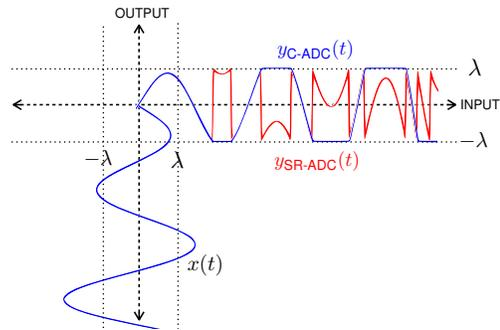
**Fig. 1.** An illustration of the transfer characteristics of a clipping-ADC and a self-reset-ADC with the thresholds at  $\pm\lambda$ .
