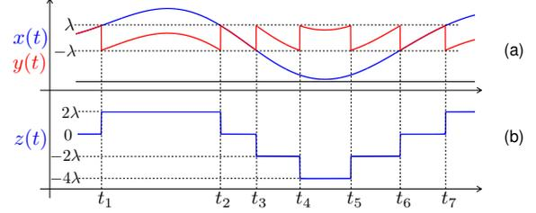
**Fig. 2.** Modulo operation: (a) Input signal  $x(t)$  (in blue) and its modulo version  $y(t)$  (in red); and (b) piecewise-constant signal  $z(t)$ .
