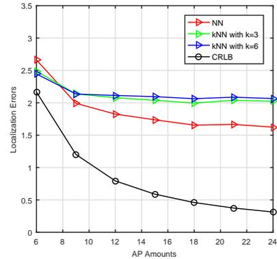
**Fig. 2.** The localization errors on different number of APs under the CRLB and the fingerprint-based approach.
