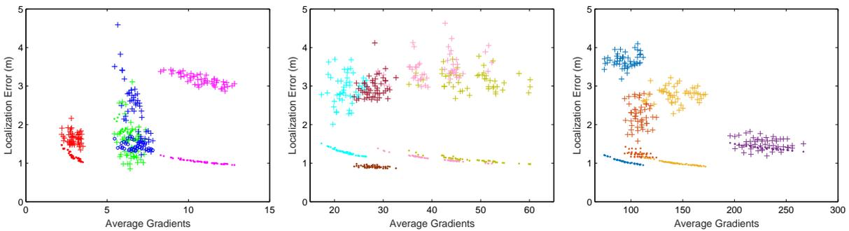
(c) The CRLB vs. the localization error using kNN with  $k = 6$ .
