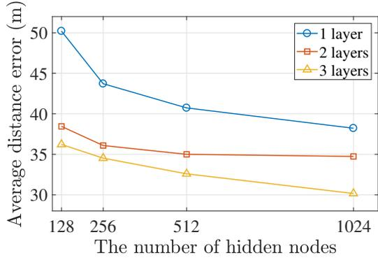
**Fig. 4.** Average distance errors for various nodes and layers.
