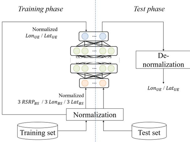
Fig. 2. Block diagram of DNN training and test.
