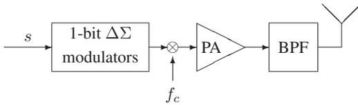
Fig. 1:  $\Delta\Sigma$ -based transmitter.
