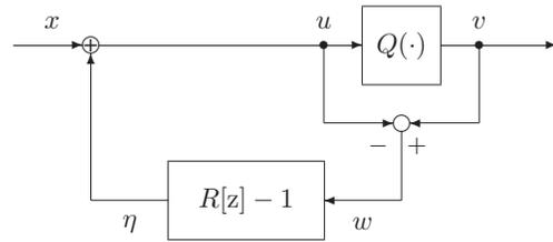
Fig. 2:  $\Delta\Sigma$  modulator.
