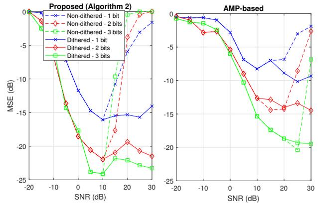
**Fig. 4.** MSE for dithered and non-dithered quantization cases.
