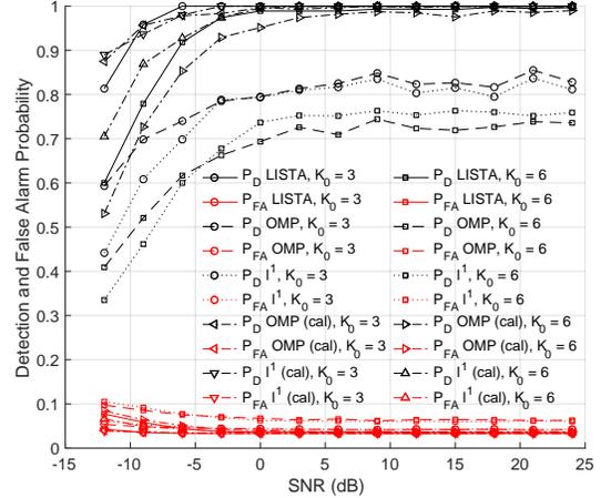
**Fig. 2.** Probability of detection and probability of false alarm plots for OMP, LISTA, and proximal gradient descent in the presence of linear nonidealities over signal SNR. For  $K_0 \in \{3, 6\}$  we plot the mean  $P_D$  and  $P_{FA}$  averaged over 200 experiments on independently-generated signals with SNR swept from  $-12$  dB to  $21$  dB in steps of  $3$  dB. Calibrated algorithms are run using unimpaired data.
