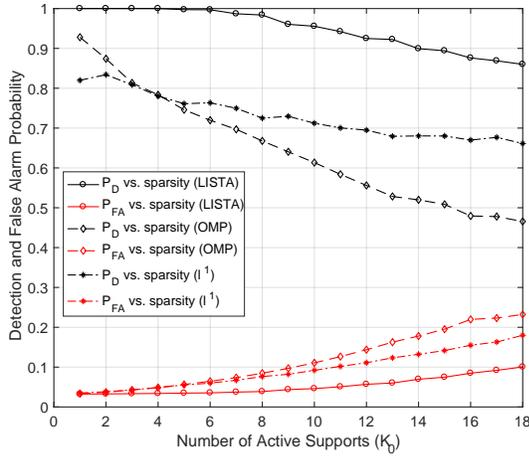
**Fig. 3.** Probability of detection and probability of false alarm plots for OMP, LISTA, and proximal gradient descent in the presence of linear nonidealities over signal sparsity. We fix the signal SNR at 20 dB and plot the mean  $P_D$  and  $P_{FA}$  averaged over 500 experiments on independently-generated signals with sparsity swept from 1 to  $R$ .
