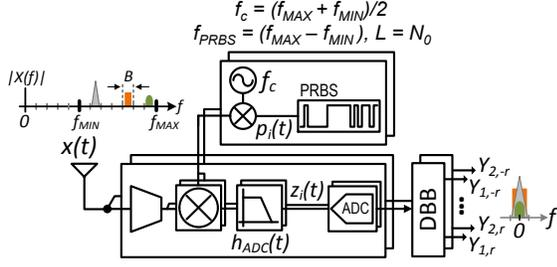
**Fig. 1.** Simplified schematic of the Direct RF-to-Information Converter.
