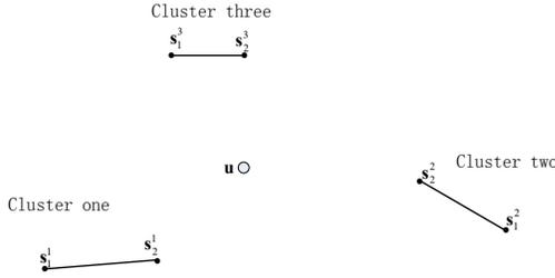
**Fig. 1.** Illustration of nodes partly synchronous TDOA source localization system, where the nodes connected by lines means they are synchronized.
