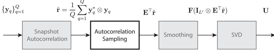
**Fig. 1.** Coprime processing steps: from a collection of samples  $\{\mathbf{y}_q\}_{q=1}^Q$  to the estimated coarray signal-subspace basis  $\mathbf{U}$ .
