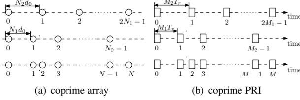
**Fig. 1.** Coprime array and coprime PRI configuration.
