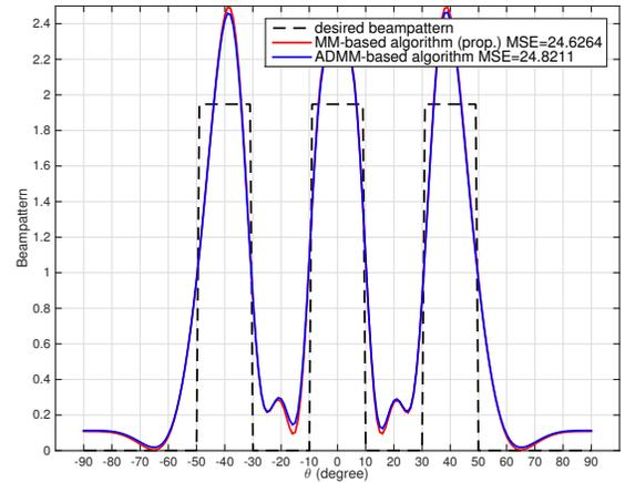
**Fig. 3.** Transmit beampattern design with 3 targets.
