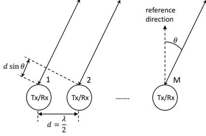
**Fig. 1.** MIMO transceiver with  $M$  antennas and  $\theta$  is the spatial direction of interest.
