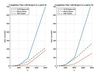
Fig. 3: Completion time of Hard and Soft Clustering methods with  $k \in \{8, 16\}$ .
