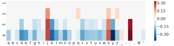
Fig. 5: Difference in accuracy of character recall between a 1-layer GRU and 5-gram trained on WSJ. Axis are the same as in Figure 4. Red cells represent stronger GRU recall, blue cells represents stronger n -gram recall.
