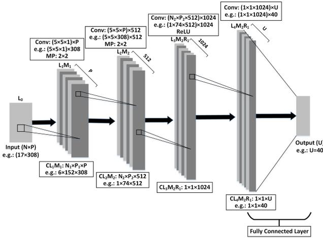
Fig. 2. Employed CNN Architecture.
